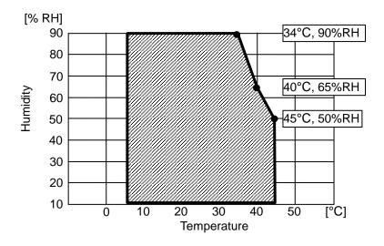
Figure 2-1 Operating Temperature and Humidity Range
