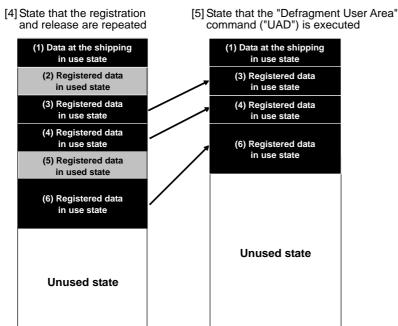
When data registration and release are repeated, the memory state turns to the [4] state in the figure. In order to use the "Used state" area again, execute the "Defragment User Area" command ("UAD"). The [5] shows the memory state after defragmented.
